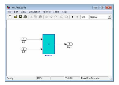
**2** Examine the model. The highlighted block multiplies two full-range signals, which could result in an overflow.
