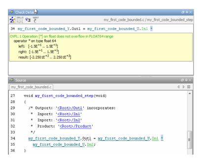
The OVFL check is now green. Polyspace verification shows that no run-time errors are present in the model.
