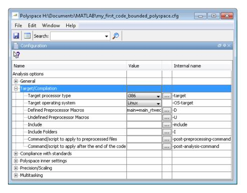
**3** The **Target processor type (-target)** option defines the size of data types.
